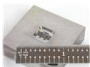
The shop's investment in the EDM and metrology system was in response to increasing demand for smaller, more complex parts, such as the medical staple mold shown here.
