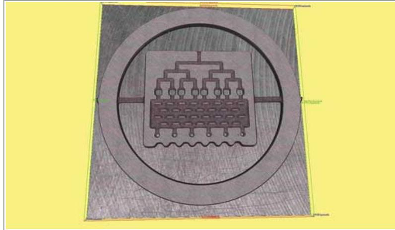
The measurement of micro-machined components has produced significant challenges for measurement and inspection. The components to be measured generally have steep slopes, complex geometries, multiple forms, and varying reflective properties; (for example, see Figure 1, below). In addition, they generally have stringent surface finish requirements.
